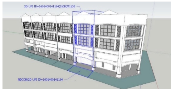
Fig. 5. Example of proposed 3D UPI (LoD3, D3) based on NDCDB 2D UPI.
